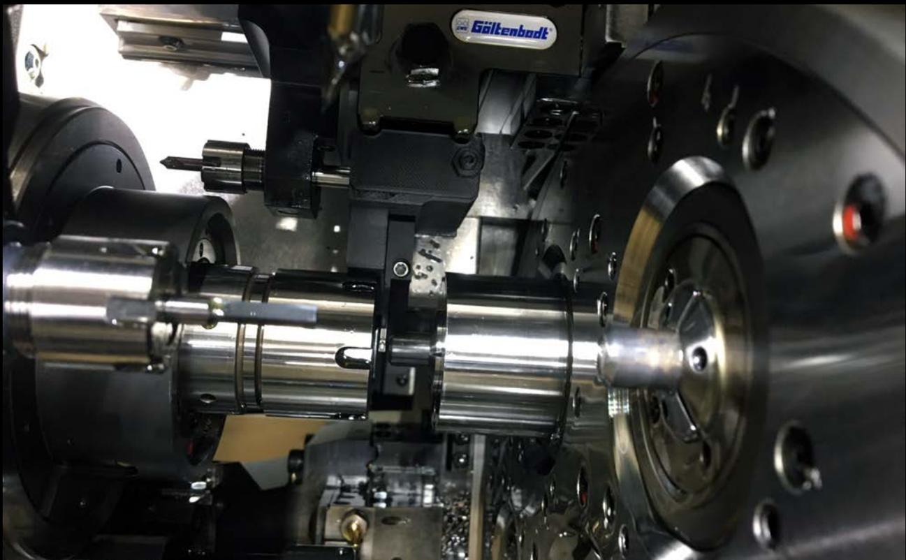
The new G80A parting-off system, also includes the details that offer added performance, reliability and efficiency. The targeted internal coolant supply makes the process even more reliable and enables longer tool life.
