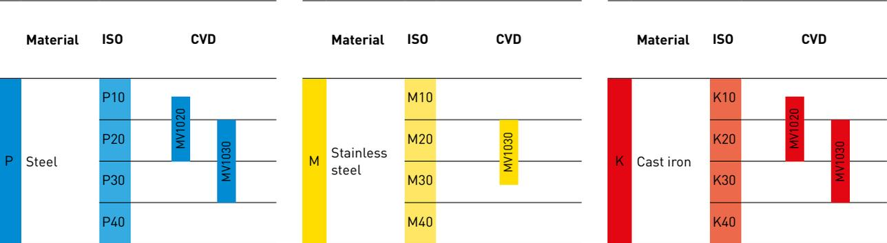
1. Dry cutting is recommended for machining stainless steel with MV1030.
