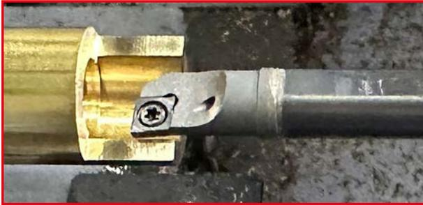
**Boring Bar for machining small parts**
