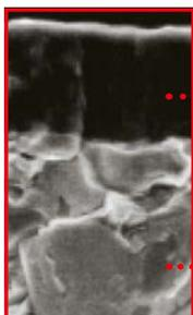
PVD coated grade suitable for a wide range of applications. The combination of a special tough cemented carbide substrate with MIRACLE coating provides an excellent balance of wear and fracture resistance.
